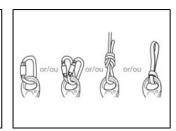
The swivel accepts up to three carabiners and allows the use of ropes and slings to facilitate maneuvers.
